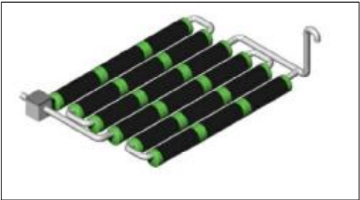
GRAVELLESS MEDIA-WRAPPED CORRUGATED PIPE SERIAL DISTRIBUTION GENERAL DETAIL
