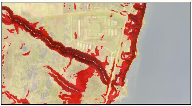
Little or no slope: 0-3% gradient Steep slopes: 16-30% gradient Gentle slopes: 4-9% gradient Extremely steep slopes: 31-60% gradient Moderate slopes: 10-15% gradient Excessively steep slopes: > 60% gradient
