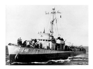
The PC-461 class were a class of 343 submarine chasers built mainly for the US Navy and built from 1941-1944.
